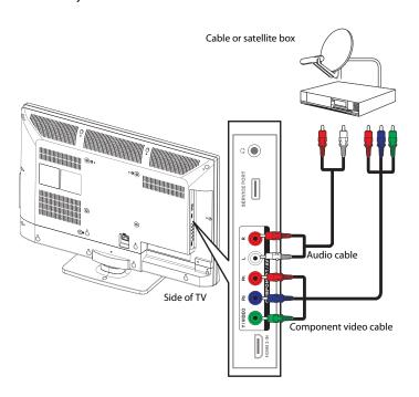
4 Connect an audio cable (not included) to the L and R audio jacks on the side of your TV and to the audio out jack on the cable or satellite TV box.
